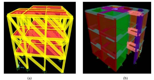
Figure 2. SAP model of the study building: (a) RC frame with masonry infill by equivalent strut (b) confined masonry wide column model
