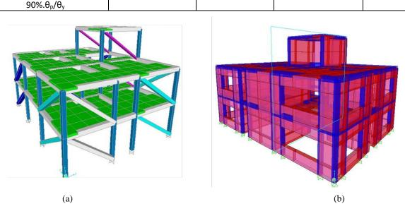
Figure 5. SAP models of Building 2: (a) RC frame with masonry infill (b) confined masonry
