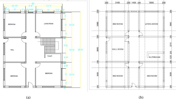
Figure 4: Floor plan of Building 2: (a) Original RC frame with infill (b) Equivalent confined masonry
