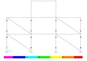
Figure 7. Hinge formation in the frame of RC buildings with infill
