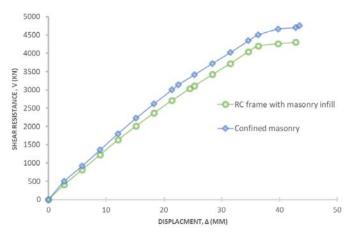
Figure 6. Static non-linear push over curve for RC frame infill and confined masonry models of Building 2
