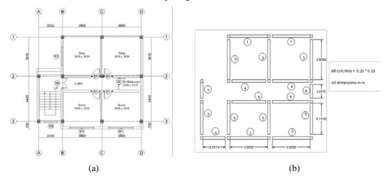
Figure 1: Floor plan of Building 1: (a) Original RC frame with infill (b) Equivalent confined masonry
